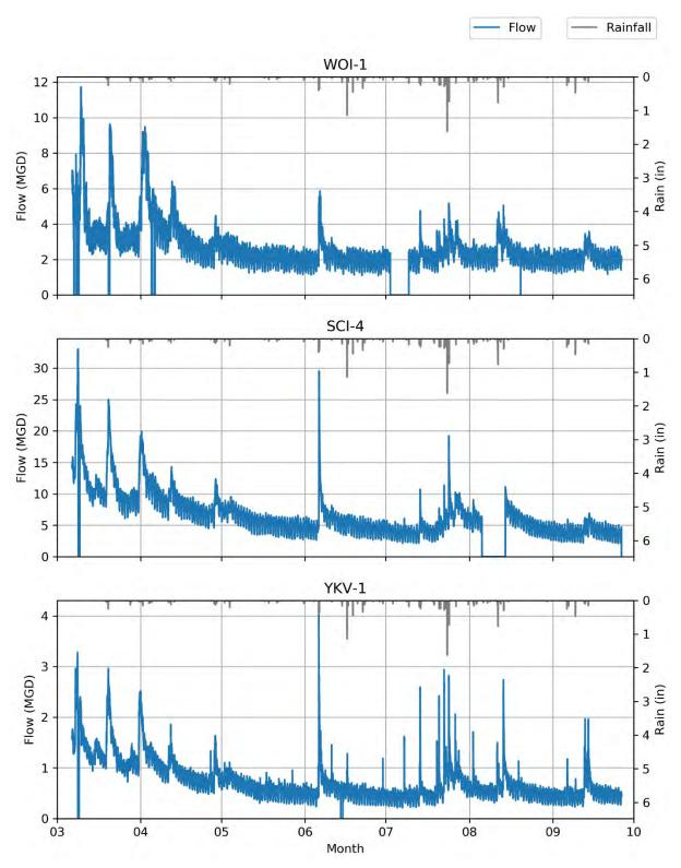
Figure 3-6. Flow Meter Data upstream of the SCPS during 2008
