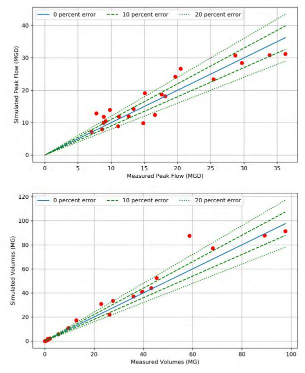
Figure 4-2. Pre-Rehabilitation Model Calibration Results for Rain Events
