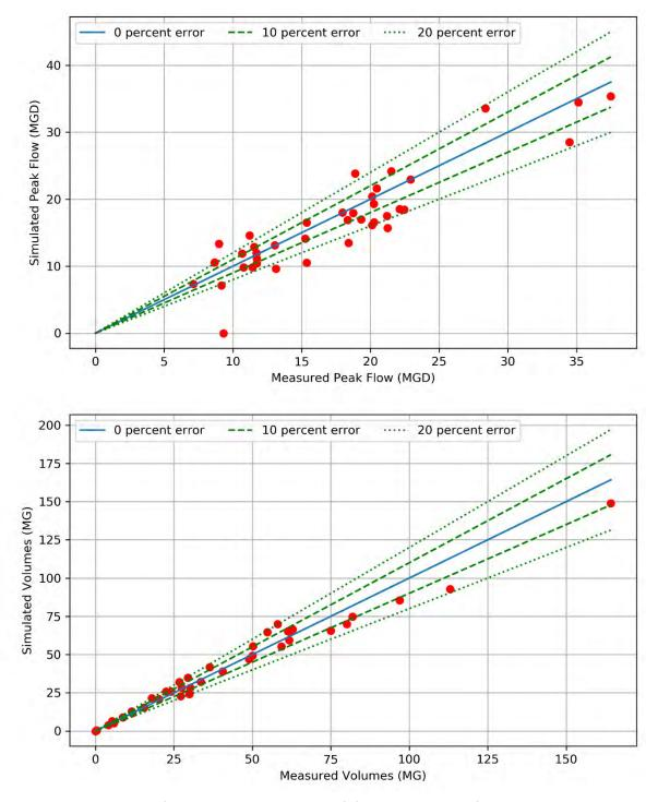
Figure 4-6. Post-Rehabilitation Model 2 Calibration Results for Rain Events
