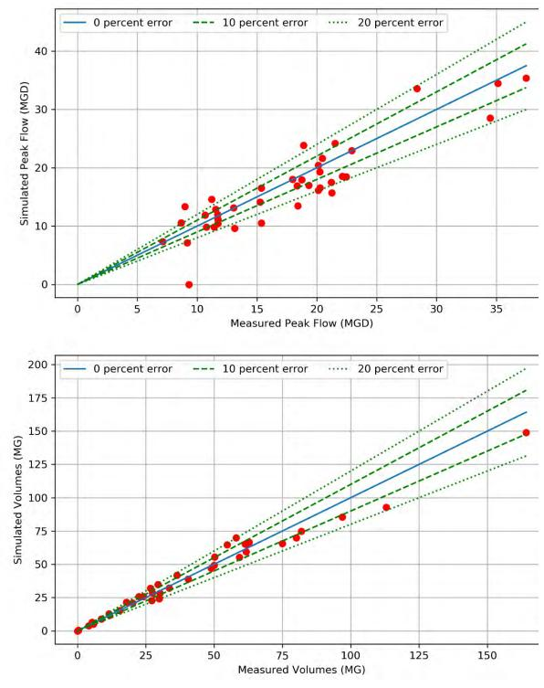
Figure 4-4. Post-Rehabilitation Model 1 Calibration Results for Rain Events
