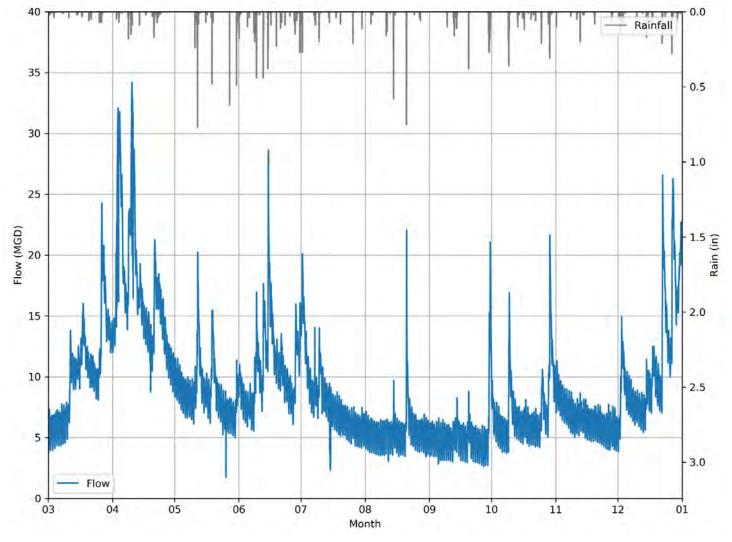
Figure 3-11. Total Flow into the SCPS during 2015
