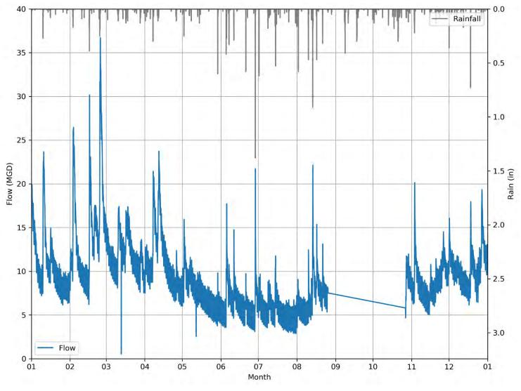
Figure 3-12. Total Flow into the SCPS during 2016
